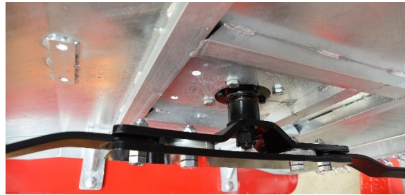
Double plate cutterbar with round swing back stop. Grade 12.9 M20mm standard bolt and Nyloc nut hardware
