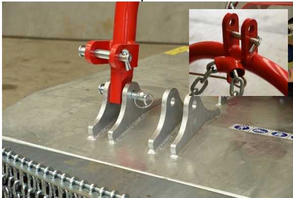
Two position headstock offset with pin. Auto-centering chain on headstock.
